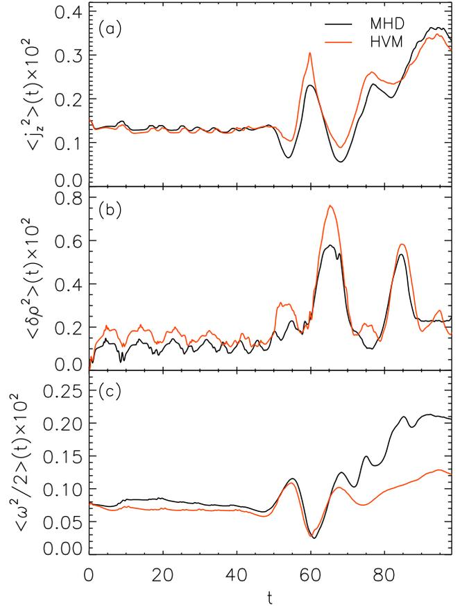
**Figure 3.** Temporal evolution of  $\langle j_z^2 \rangle(t)$  (a),  $\langle \delta \rho^2 \rangle(t)$  (b), and  $\langle \omega^2 / 2 \rangle(t)$  (c) for the MHD (black line) and HVM (red line) simulations.
