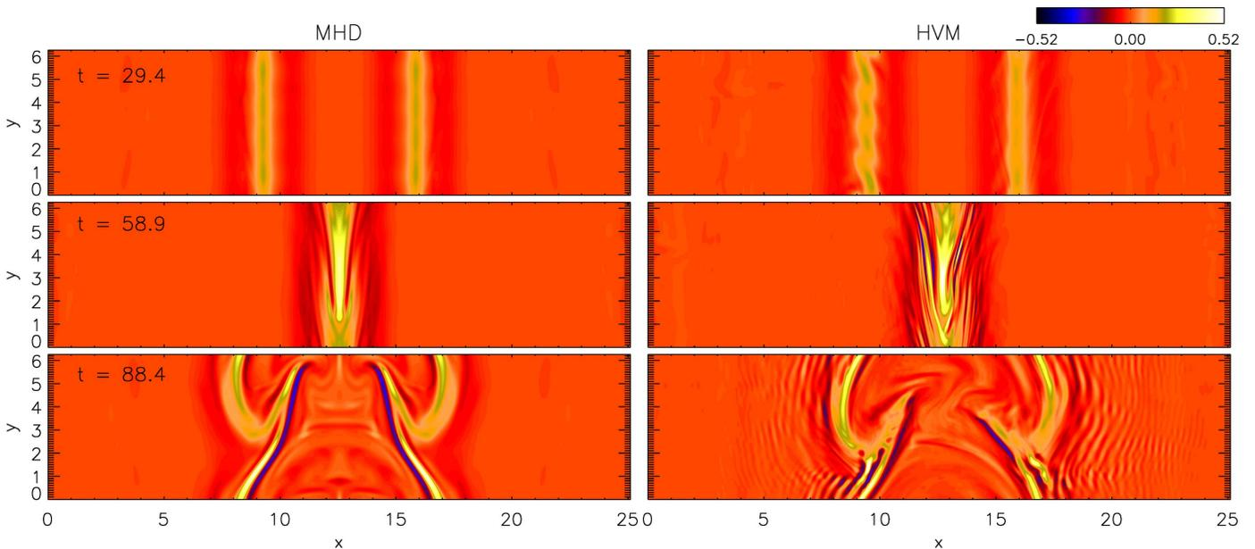
**Figure 1.** Contour plots of the current density  $j_z(x, y)$  for the MHD (left) and the HVM (right) simulations. Top, center, and bottom rows correspond respectively to the time instants  $t = 29.4$ ,  $t = \tau = 58.9$ , and  $t = 88.4$ .
