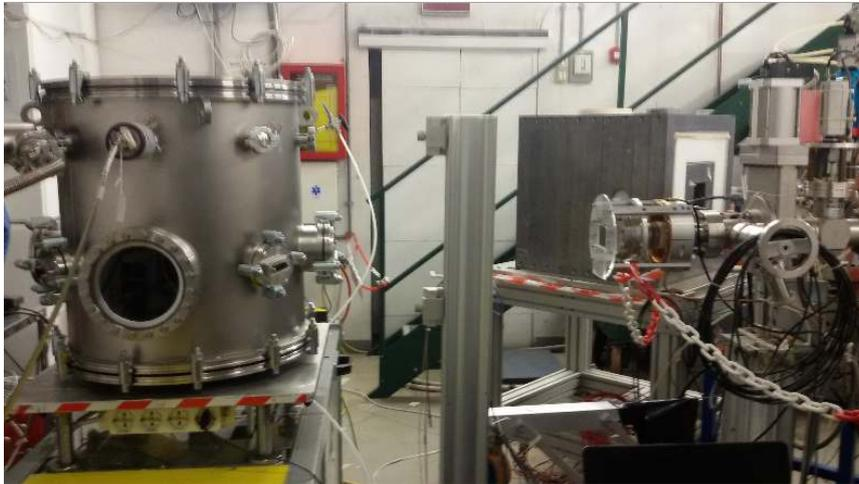
**Figure 2.** Experimental setup at the BTF, with the electron beam going from right to left into the vacuum vessel (cylindrical stainless steel container on the left).
