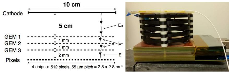
**Figure 1.** NITPC detector: on the left a schematic showing the distances between the cathode, the GEMs and pixels planes, and on the right a picture showing the full detector, with the field cage polycarbonate field rings in black and the PCBs composing the GEMpix below.
