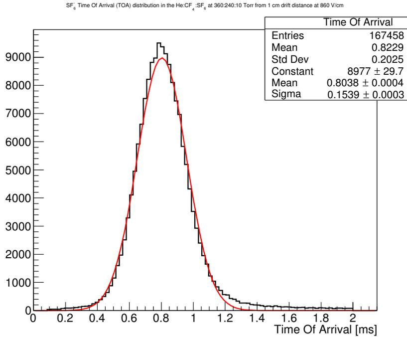
**Figure 3.** Example of the gaussian fit to the time of arrival distribution of the ionization cloud for the He:CF<sub>4</sub>:SF<sub>6</sub> 360:240:10 Torr mixture at 1 cm drift distance with a 860 V/cm drift field.
