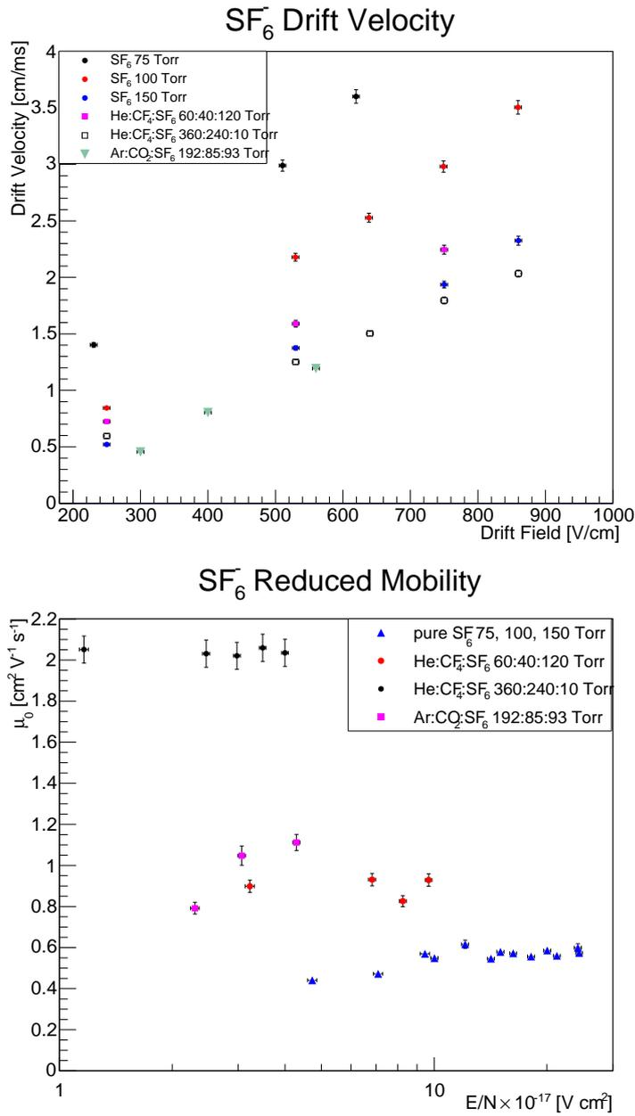
**Figure 5.** SF<sub>6</sub><sup>-</sup> drift velocities (top) and reduced mobilities (bottom) in pure SF<sub>6</sub> (at 75 Torr, 100 Torr and 150 Torr), in Ar:CO<sub>2</sub>:SF<sub>6</sub> at 192:85:93 Torr and He:CF<sub>4</sub>:SF<sub>6</sub> at 60:40:120 Torr and 360:240:10 Torr.
