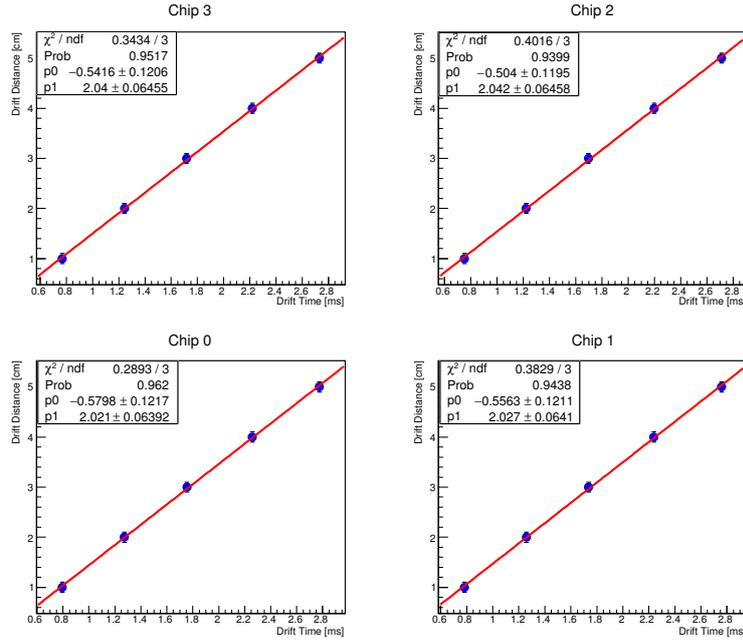
**Figure 4.** Chip by chip fit of the TOA versus drift distance, in order to extract the drift velocity of  $\text{SF}_6^-$  in  $\text{He}:\text{CF}_4:\text{SF}_6$  360:240:10 Torr ( $p_1$  fit parameter).
