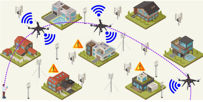
Fig. 1. Our envisioned scenario involves an operator or a central unit piloting UAVs in BVLoS. The operator has limited visibility and follows the drone using the cellular infrastructure. The drone's path is selected by prioritizing robust wireless connections and ground safety.
