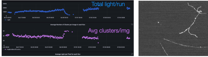
Figure 3.18: On the left an example of two variables of the slow control which check the quality of the data captured with the sCMOS camera. Occurrences of issues was notice by the slow control during this initial test phase. On the right, an example of an image from the sCMOS camera taken on LIME at the underground laboratories of LNGS.
