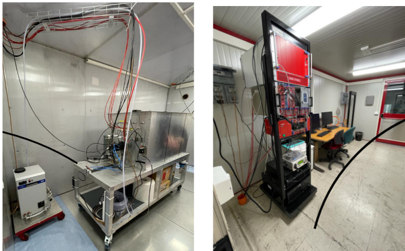
Figure 3.17: Pictures of the ground floor (left) and the first floor (right) with respectively LIME detector inside its Faraday cage and the control room.
