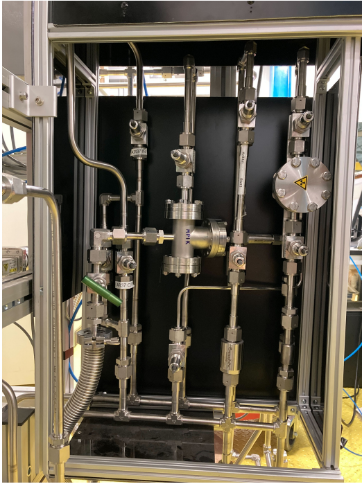
Figure 5.4: (Credits to Florian Jörg, March 2023) XENONnT calibration system source box, with the ^{222}\text{Rn} emanating sample (in the center of the picture) just installed by Florian Jörg, Ying-Ting Lin and the author.
