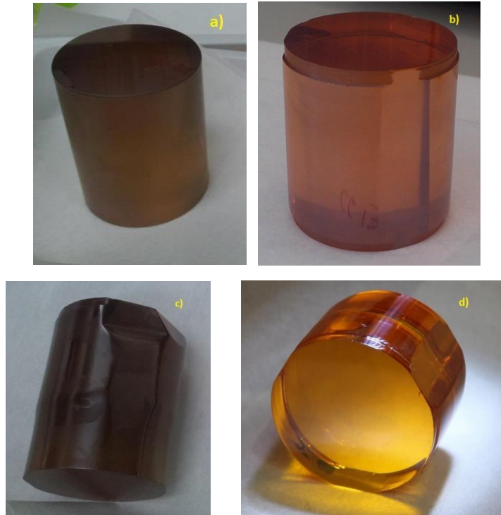
Figure 3.8: Zn 82 Se crystals of different shape ready for mounting: a) perfect cylindrical shape; b) collar and lateral strip aimed at fitting the copper frames; c) dedicated cut for maximum mass; d) short crystal.
