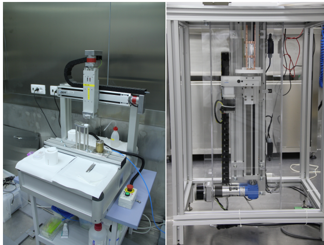
Figure 3.28: Photos of the two working areas inside the cleanroom. On the left is shown the station where the Ge-NTD thermal sensors are glued to the absorbers, on the right is shown the area where the towers are assembled and stored.
