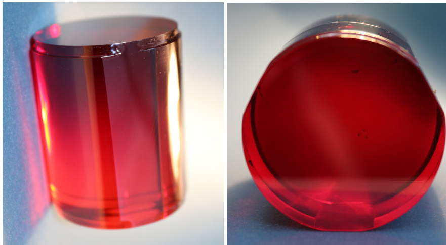
Figure 3.19: Picture of the two enriched crystals (CG-28 on the left and CG-29 on the right) not used in the analysis due to their poor bolometric performances. Usually ZnSe crystals are orange while they are red.
