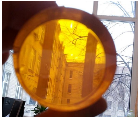
Figure 3.13: Optically polished \text{Zn}^{82}\text{Se} crystal.
