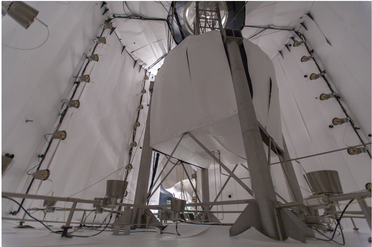
FIG. 14. View of the inside of the WCV of the DarkSide-50 detector. The stainless steel sphere of the LSV at the center of the water tank is shown covered with its Tyvek reflector. PMTs are mounted on the wall and floor of the WCV.
