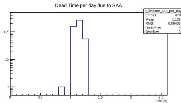
Figure 3.5: Daily contributions subtracted from the total livetime, due to the passage through the SAA region. From [69].
