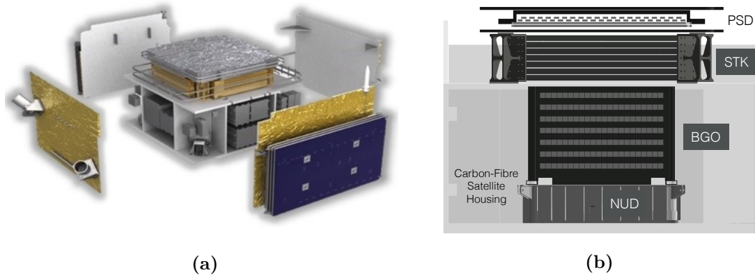
Figure 2.2: The complete DAMPE payload in its (a) exploded view along with (b) a cross-section illustrating its various sub-detectors. From [63].
