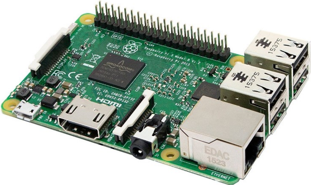
FIGURE 5.3: Raspberry PI 3 Model B with 1.2 GHz Quad Core CPU [66]
