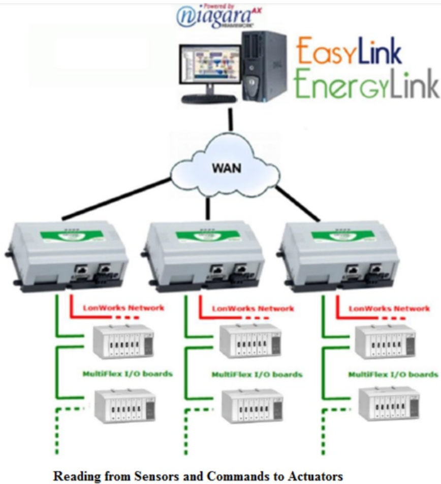
FIGURE 2.12: Process Flow Diagram from Sensors to Niagara Framework [18]
