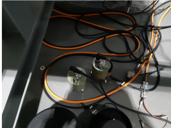
Figure 9.1: Two Trillium compact seismometers. One was connected to KAGRA’s acquisition system, while for the other one this was not possible, so it was just deployed close to the first one in order to synchronize them.
