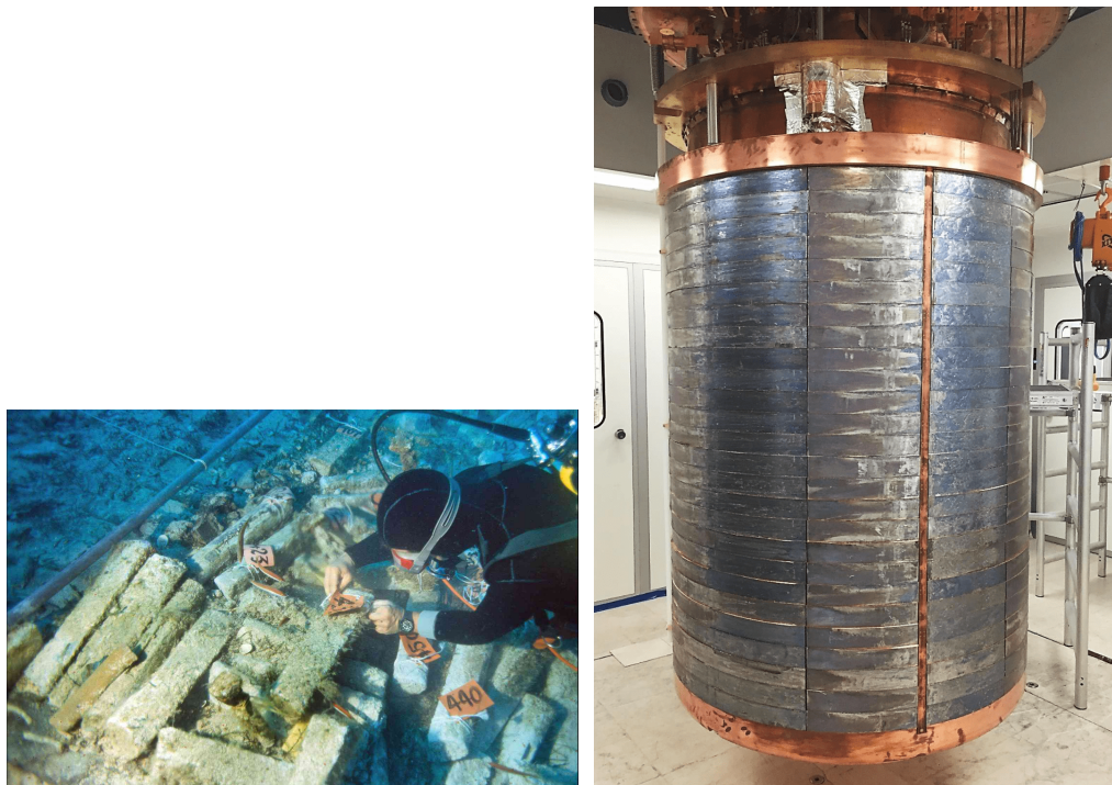
FIGURE 2.18: [Left] Recovery of the roman lead ingots. [Right] Lateral and bottom roman ILC mounted in the CUORE cryostat; the lead ingots were casted into circular sectors to build the shield structure.
