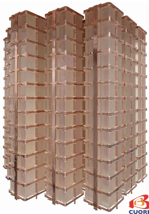
FIGURE 2.11: The complete CUORE detector: the 19 towers modules hosting the 988 TeO_2 crystal.
