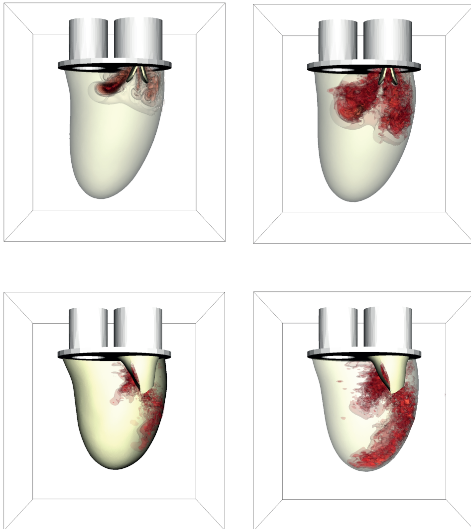
Figure 2.12: Snapshots of the flow inside the ventricle at the two different time instants (left and right panels) in the diastolic phase of the cardiac cycle. Top panels show the ventricle with a mechanical natural valve while the bottom panels show the ventricle with a deformable natural valve. The colour represents the iso-surface of the velocity magnitude of the flow inside.
